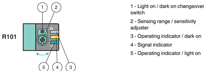
To unlock the adjustment functions turn the sensing range adjuster for more than 180 degrees.
